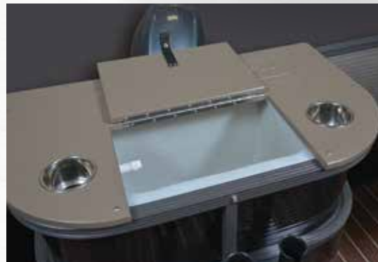
Stern fish area with 10 gallon livewell & rod holders.
